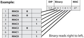
"MACO" refers to the first bit in the binary string, from there the dip switches are set following the description ordering using the binary string for the desired setting.
