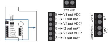
Outputs 1(V1,I1), 2(V2,I2) and 3(V3,I3), will be auto populated in order of the AQ2W ordering matrix: CO2, RH, Temp, VOC, PM, Slider, CO, O3
