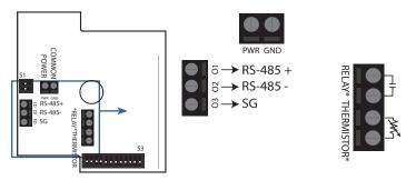
NOTE: A 120  $\Omega$  termination resistance may be added in parallel with the RS-485 +/- by moving the very top DIP switch (DIP 1) to the left position. See "DIP Configuration" section for more information.
